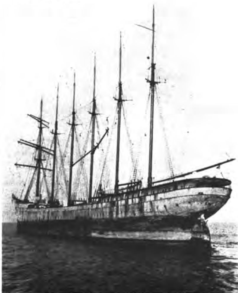
The world has only known two six-masted barkentines. One was the City of Sydney , built in 1875 as an iron-hulled steamer for the Pacific Mail Line. In 1916 her hull was purchased by L. A. Pedersen of the Bristol Bay Packing Company, who converted her to the sail rig shown above. From 1918 until 1924 she was used in the Alaska salmon trade and was finally broken up for scrap in California.
